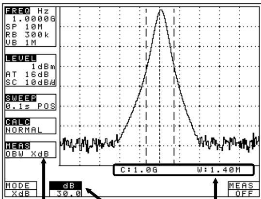
[Occupied frequency bandwidth measurement mode]      [Parameter]      [Measured value]
